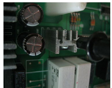
Typical PCB Ground REG1 Heater Sink
